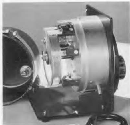
Figure 2. Interior view of the Type 1215-A Unit Oscillator with shield cover removed.
